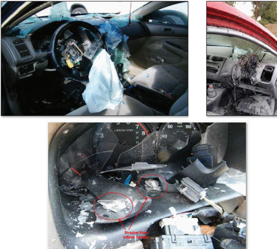
Figure 2: Photographs of Vehicles with an Exploded Driver-Side or Passenger-Side Defective Takata Airbag Inflator
